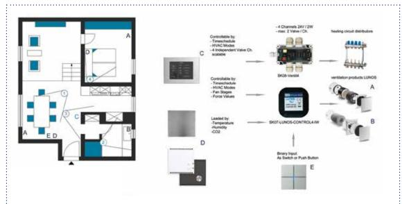
A = LUNOS  $e^2$  Set • B = RA 15-60 Exhaust • C = Touch-IT / C3 / Smart / NEO • D = Sensors: temperature, humidity, CO<sub>2</sub>, SK30-THC-CO<sub>2</sub> / NEO-THC-CO<sub>2</sub> / E = Various switch systems
