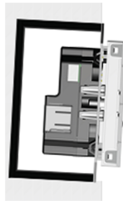
Flush-mounting incorrectly installed
