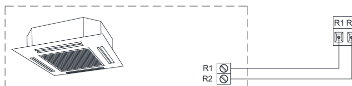
Figure 2: Wiring KLIC-PA to the Air Conditioning Equipment
