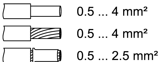
Figure 2: Clampable conductor cross-section
