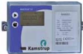
MULTICAL 62 is an ultrasonic flow sensor, used for measurement of cold (0.1...50°C) and hot water consumption (0.1...90°C) in commercial, industrial and residential buildings. The ultrasonic sensor does not include any mechanical parts, avoiding deterioration and therefore extending its life time. The meter keeps its precision, also for low flows, during its total lifetime. The KNX module is directly plugged into a slot on the meter. The meter is MID approved.
