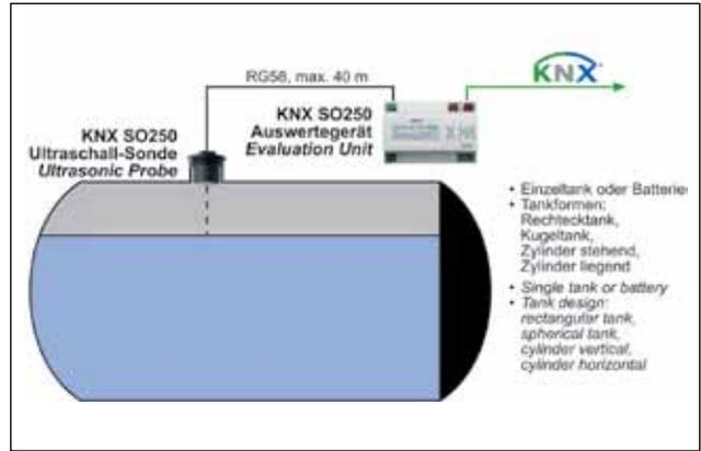
The tank probe KNX SO250 of Elsner can be used to measure distances and check volumes in containers. It consists of an output device and an ultrasonic probe, with a range of 12 to 250 cm. The KNX SO250 has a connection to KNX and two additional outputs that can be switched when exceeding or dropping below a specified volume or distance. For this, the
