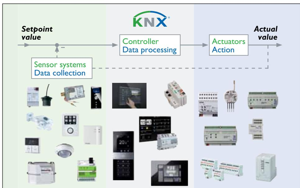
KNX sensors, meters and actuators
