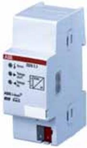
The meter interface Module ZS/S 1.1 allows registering and transmitting meter data and values from energy meters to KNX. The device contains an infrared interface, which supports ABB meter types DELTAplus, DELTAsingle, ODIN and ODINsingle or the new energy meters of the A-series. The read information can be used for example for cost-centre accounting, energy optimization, visualization or the monitoring of installations.
