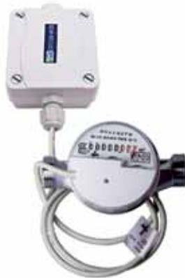
The In Home water meter is a combination of the calibrated water meter 'Modularis WZ-M' from NZR and the impulse counting unit SK01-IMPZ1 from Arcus-EDS GmbH, the latter including a battery buffered data storage and KNX bus coupling unit. In this way, the product can be used for remote reading and monitoring.
