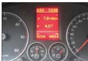
Indicazione del consumo istantaneo in auto / Fuel consumption indicators in cars
