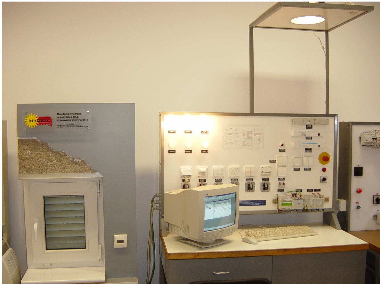
Fig. 2. View of the EIB-TP lab stand.
