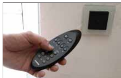
Figure 2. All the building services can be comfortably controlled with the KNX RF remote control.
