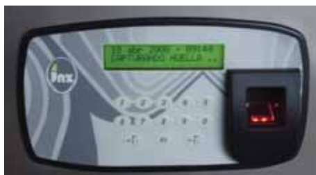
Picture 2. Thanks to the interface of the access control system (finger print) to the KNX system, a customized control of all systems is possible.
