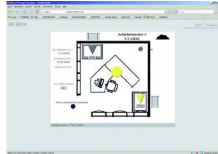
Figure 6. The operating interface for room automation communicates with the KNX system via Web technology. Source: Kuhlmann
