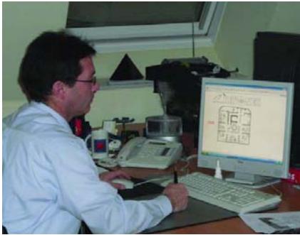
Figure 5. Lighting, shading, window ventilation and heating can all be operated from any workplace PC. Source: Kuhlmann
